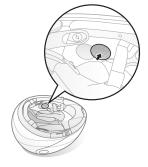
6. Insert the control buttons and microphone unit between the external shell and the left inner shell. Click the snap through its snap holder.
