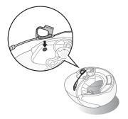
7. Hide the wires behind the center pad and reinstall the cheek pads. Make sure to click the snaps through the snap holders.
