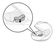
7. Hide the wires behind the center pad and reinstall the cheek pads.
