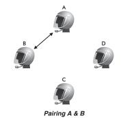
4. You can make other pairing between headsets A and C, and between headsets A and D by following the same procedure as above.
