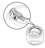
4. Slide in the antenna between the external shell and the left inner shell. Align its snap holder with the bottom left snap.
