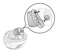
7. Attach the speaker and put the cover back on. Go through the same process for the other cheek pad.
