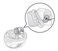
8. Place the FM antenna between the outer shell and the comfort lining around the top shell of the helmet. Make sure the end of the FM antenna is placed at front left part of the helmet away from the antenna.
