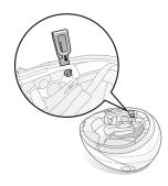
3. Insert the main unit between the external shell and the inner shell. Align its snap holders with the rear snaps.
