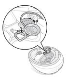
Insert the headset buttons and microphone unit between the external shell and the left inner shell. Align its snap holder with the front left snap.
