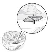
Peel off the cover of the adhesive tape of the hook and loop fastener for microphone and attach it on the inside of the helmet's chin guard. Attach the wired microphone on the hook and loop fastener and insert the microphone cable into the microphone connector.
