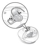
6. Insert the headset buttons and microphone unit between the external shell and the left inner shell. Align its snap holder with the front left snap.
