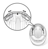
4. Peel off each cover of the hook and loop fasteners for speakers to expose the adhesive surface. Then, attach the fasteners to the ear pockets inside the helmet.
