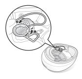
3. Unfasten the two snaps of the center pad in the back and insert the battery unit between the external shell and the inner shell. Click the two snaps through the snap holder of the battery unit.
